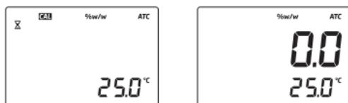
4. Gently absorb the ZERO water standard with a soft tissue. Use care not to scratch the prism surface. Dry the surface completely. The instrument is ready for sample measurement.
