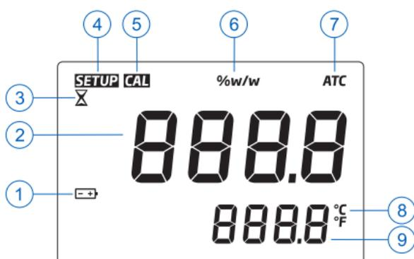
1. Battery (blinks when low battery condition detected)
