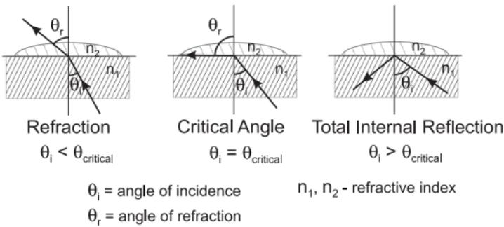
In the [HI96804](#), light from an LED passes through a prism in contact with the sample. An image sensor determines the critical angle at which the light is no longer refracted through the sample. The [HI96804](#) automatically applies temperature compensation to the measurement and converts the refractive index of the sample to Invert Sugar concentration in units of percent (by weight).
