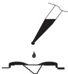
3. Press the **READ** key. The result is displayed in units of % by weight (% w/w).
