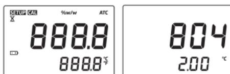
2. While continuing to hold the **ON/OFF** key, press the **ZERO** key. The temperature unit will change from  $^{\circ}\text{C}$  to  $^{\circ}\text{F}$  or vice versa.
