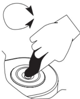
2. Using a plastic pipette, drip sample onto the prism surface. Fill the well completely.
