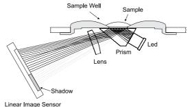
Specialized algorithms then apply temperature compensation to the measurement and convert the refractive index to: g/100 g (% by mass), g/100 mL, Specific Gravity (S.G. 20/20) or °Baumé.
