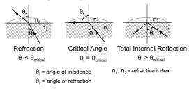
In the H196821, light from an LED passes through a prism in contact with the sample. An image sensor determines the critical angle at which the light is no longer refracted through the sample.
