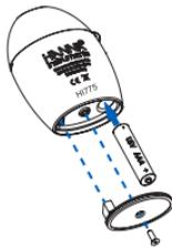
3. Remove the old battery, replace it with a new 1.5V AAA battery, inserting the negative end first.
